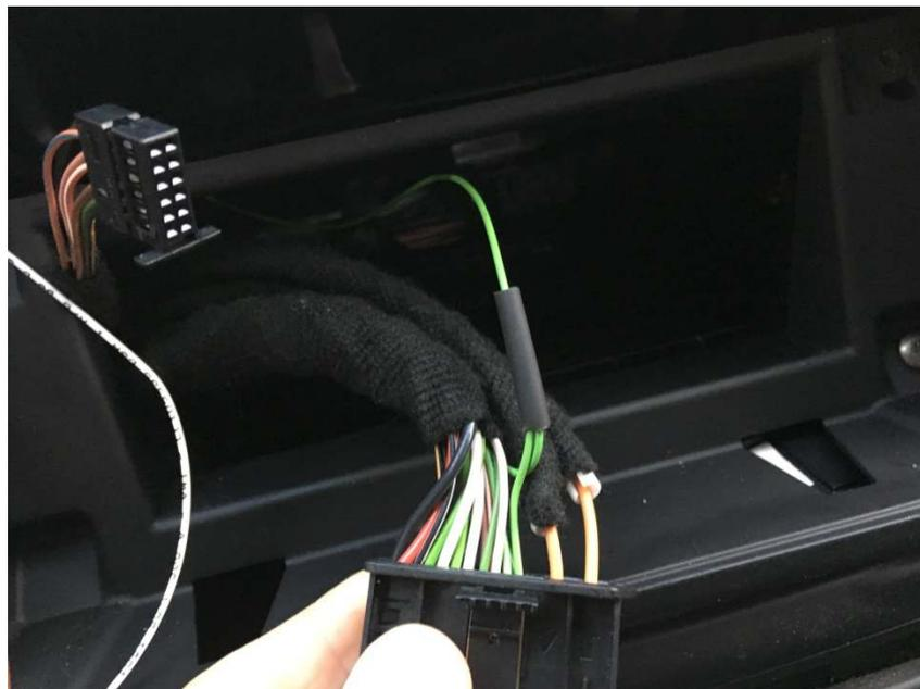
Step 14) Move the SID connector housing that was removed in the earlier step and attach it to the short adapter cable that will be placed between eSID-HPD and SID. It shall be put on the side where the connector is NOT cut.
