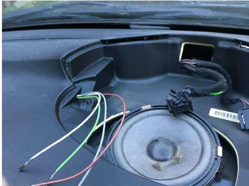
Step 7) Remove the connector housing to the SID (will be used later for adapter cable between eSID and SID. It's a tricky connector (crap design actually). The inside part needs to be slid out and there are two small hooks that holds it in place, one on each side
