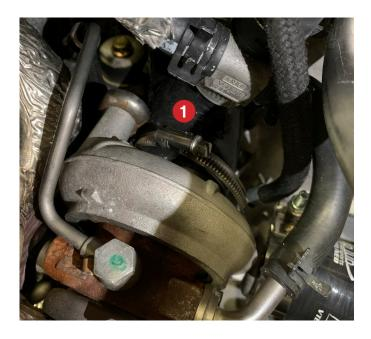
The picture shows how the intake hose is connected to the turbo.
