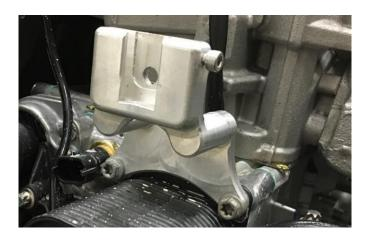
Install VICTORY mount on engine with screws from exhaust manifold.
