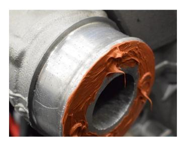
Put SUPRA COPPER on exhaust neck flange before installing it on exhaust manifold.
