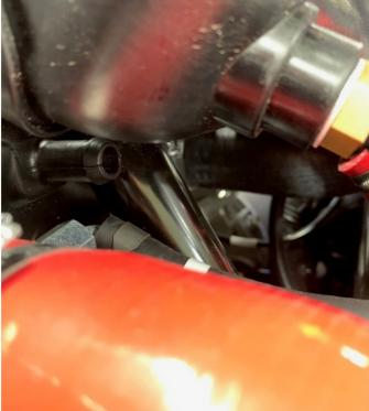
Install the straight connector in the shortened hose and connect the longer hose to the connector on the plastic intake pipe.
