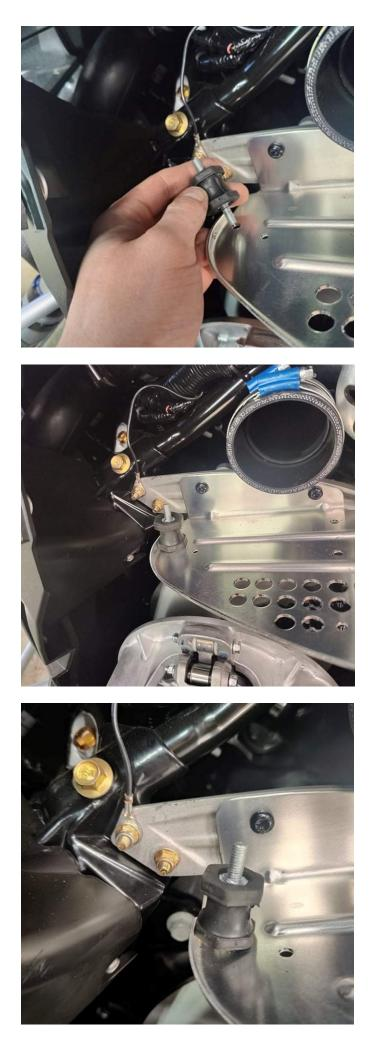
Attach the other clamp over the silicone and mount the CAI pipe in the hose, do not tighten the hose until the pipe is correctly adjusted. Install the pipe so that the lower mount fits on the installed rubber mount on the clutch protector plate. Fasten the CAI pipe with the other nut on the rubber mount and tighten the clamp on silicone hose.
