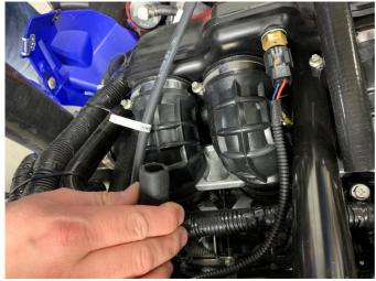
Locate a connection on the plastic intake pipe covered by silicone hat, remove the hat.
