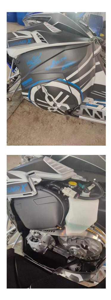
Remove air filter box according to manufacturers instructions, remove the screw on the clutch protector plate.
