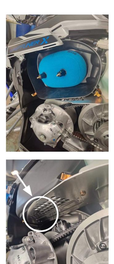
Install the aluminium ring in the plastic intake pipe and attach the silicone hose over it, fasten the hose with the included clamp.
