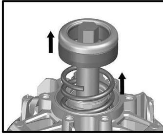
Remove spring cup, install spring after installation of clutch weights
