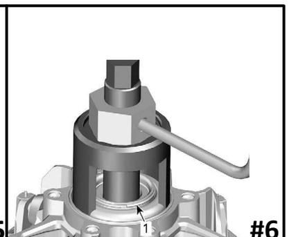
Remove Circlip #1
