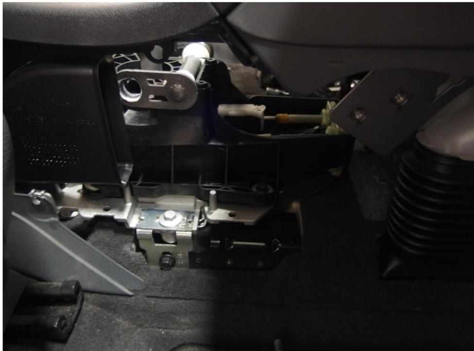
Remove four screws holding gear lever in place.
