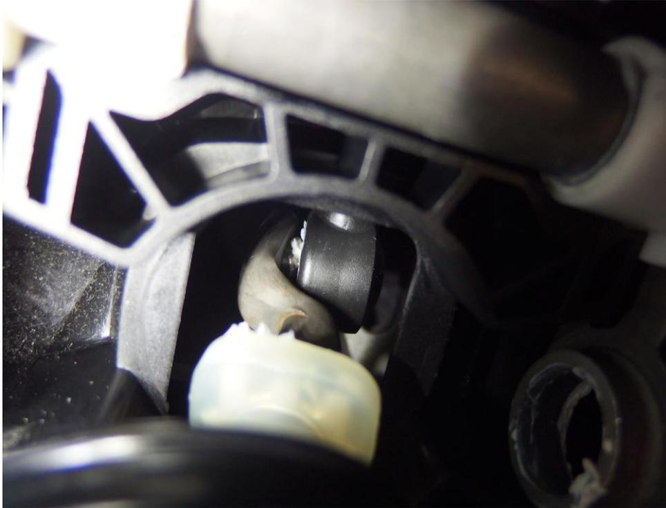
Use a screwdriver to remove lower shaft from the joint.
