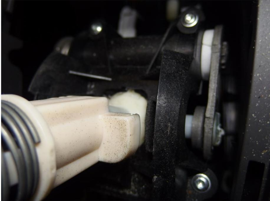
Remove 4 screws holding gear lever in position.
