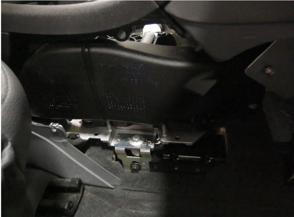
Remove AC tunnel for easy access.
