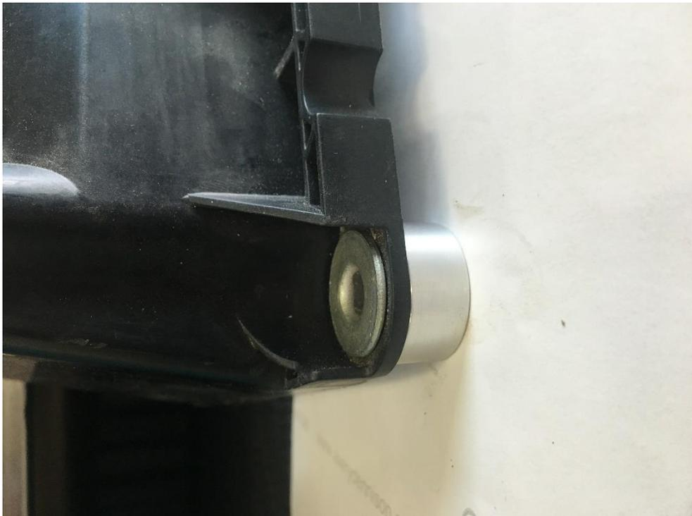
Place bushings between and use standard screw and spacer.
