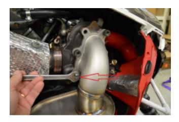
Step 8 Install and tighten the bolt for the upper bracket and use the washer that was included with the hardware.
