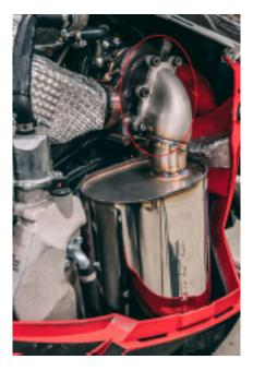
Step 10 Re-install the factory heatshield and all the plastics
