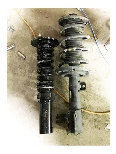
Before installation on the car, the spring must be adjusted to a default setting. Unscrew the lower spring seat (pos. A) so that the spring just makes contact with the upper and lower spring seats. After this, the lower spring seat is screwed up 5mm to get the correct pretension on the spring.
