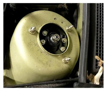
t this point you will want to adjust the collar/bracket for ne sway bar link. Make sure that this collar/bracket is s high up as possible agains the spring seat. See photo ith illustration (1).
