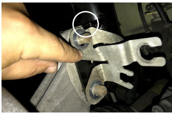
After fitting the notched out bracket tighten the nuts down and then add in the wheel speed sensor wiring then the brake hose with the clips removed from the factory strut.
