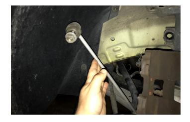
Next remove the brake line hold down and the wheel speed sensor wiring. You can use an angle pliers on all of this including the plastic hold down for the wheel speed sensor. Gently pull that off since it will be reused.
