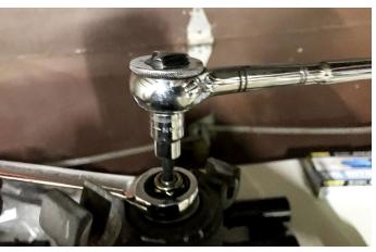
Once this is complete you're ready to reinstall the rear shock. Take the rear shock and cut the zip tie on the botom. DO NOT LOSE, DAMAGE OR MISPLACE the other half of the busing that comes out - its a two part bushing and must be installed that way. First attach the mount to the body and tighten down - then reinstall the bottom of the shock to the lower control arm.
