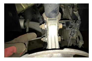
At this point you can remove the 3 bolts from the top and remove the strut.
