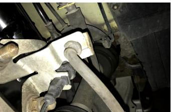
Once the brake hose and speed sensor wiring are back in place take the sway bar end link and line it up with the mount. Take the link and tighten it down then snug the set screw up. The set screw does not have to be cranked down, it just needs to be snugged up as to not cause damage to the threads.
