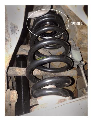
Now that you've installed the spring you can concentrate on installing the rear shock. First off remove the stock shock from the upper mount - unless this is cracked or damaged. If the upper mount is cracked or damaged replace it.
