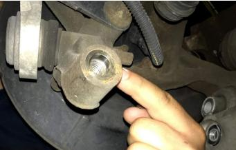
Next remove the bolt holding the lower control arm to the knuckle. SUPPORT THE CONTROL ARM WITH A JACK since this will be under pressure (the spring is already removed in the picture below. After this bolt is out you will be able to lower the jack (SLOWLY) and then remove the spring by pulling down the arm.
