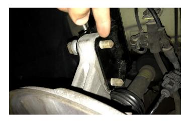
After this grab your new brake hose/wheel speed sensor wiring bracket and the paint marker. You will have to take this and line it up then notch it out to fit in the right area of the Maptun XT Series strut flush.
